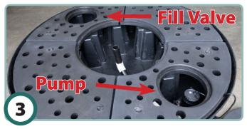
Install all basin grates, except for the grate that goes over the pump (do not install until step 6) and the center grate that is under the bowl. Be sure to install one of the grates with access port over fill valve.
