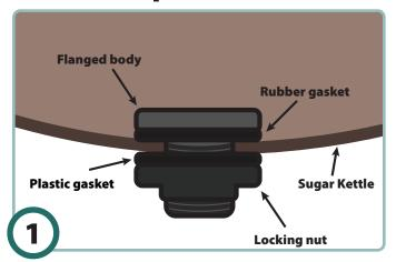
Safely lift and secure the kettle in an upright and level position. Install the bulkhead in the bottom of the kettle as shown.
