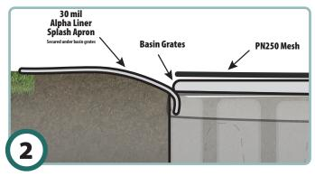
Install splash apron liner around basin. Pitch the liner towards the basin to allow splash to flow back into the basin.
