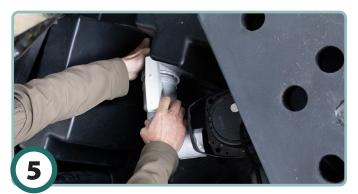
Lower the kettle until it is almost in its final position, connect the plumbing assembly to the pump outlet assembly.
