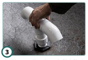
Thread the tee assembly into the top side of the bulkhead inside the kettle. Finger tighten only, **do not over tighten!**
