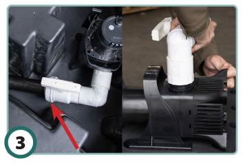
Remove plumbing assembly from pump outlet assembly using the union on the ball valve. (See photo above) Thread outlet assembly to pump. Finger tighten only, do not over tighten!
