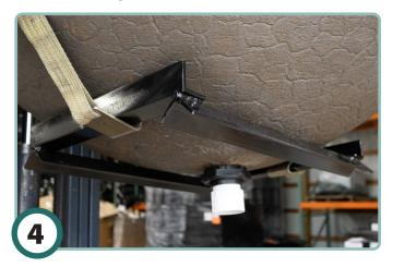
Secure the cradle stand to the bottom of the kettle using a strap to temporarily hold in position.
