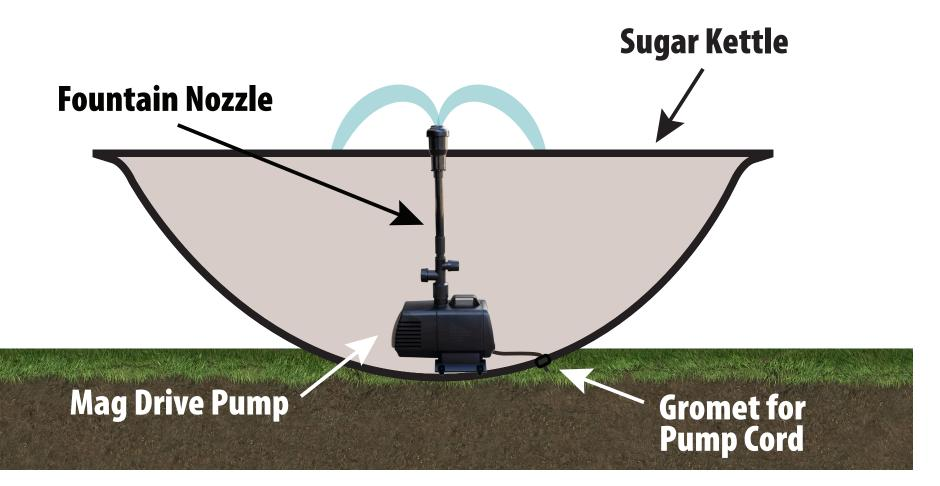
Place the pump in the kettle and use the cord grommet to bring the pump's cord outside of the kettle If you have selected the optional lighting package, install the lights in the kettle and use the cord grommet to bring the light cords out of the kettle refer to the manual included with the lights for further operation and installation instructions
